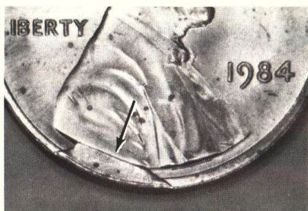
Figure 5: The cracked portion has broken away from the die that struck this cent, resulting in a cud.
